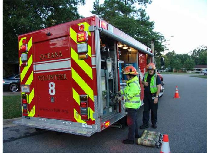
The Oceana Volunteer Fire Department, Battalion 30, has in service a 2008 International, 9 bay support vehicle designed to support emergency scene operations with a wide assortment of salvage, overhaul, SCBA air management, positive pressure ventilation/attack, lighting, and firefighter rehabilitation equipment.
