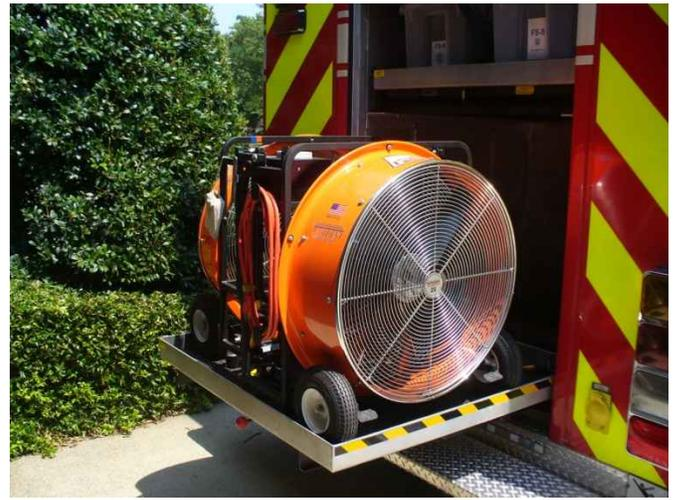
Support 8 has two 24” Tempest Variable Speed (VSX) electric fans. Utilizing intelligent drive technology, they are currently the highest rated (15,663 cfm at 2,161 rpm) of any variable speed electric fan, and can be made available for any PPV or PPA use.
