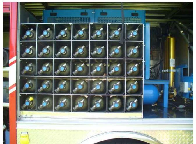
An on-board air compressor coupled with a 4 cylinder cascade system and 65 spare air cylinders allow for continuous refilling of, and a readily available cache of SCBA cylinders being available for emergency scene operations.
